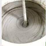
The powder component is mixed with 7 – 7.5 liters of potable water in a clean mixing container. Continually mix with a slowly rotating mechanical stirrer while adding the powder.
