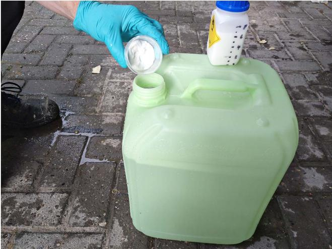
All gel times with KÖSTER B+, B-component if the organic dispersion is to be used, the measured amount of salt is transferred into the canister with the KÖSTER B+ component. The mixture is made by vigorous shaking for 3 minutes. Water is not added.
